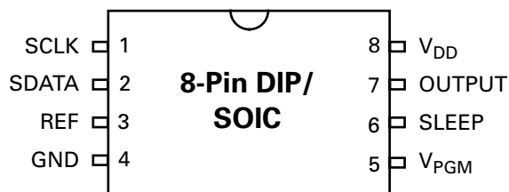
FIGURE 2. ZSBI050 8-PIN DIP AND SOIC DEVICES
