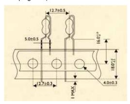
AV Type Forming for Taping (rated watts -25 & 50s & -50 & 1ws size only )
