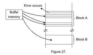
When an error happens in Block A, try to reprogram the data into another (Block B) by loading from an external buffer. Then, prevent further system accesses to Block A (by creating a bad block table or by using an another appropriate scheme).
