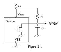
This data may vary from device to device. We recommend that you use this data as a reference when selecting a resistor value.
