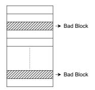
Referring to the Block status area in the redundant area allows the system to detect bad blocks in the accordance with the physical data format issued by the SSFDC Forum. Detect the bad blocks by checking the Block Status Area at the system power-on, and do not access the bad blocks in the following routine.
