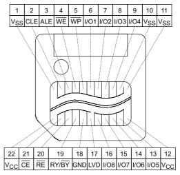
Figure 1. Pinout
