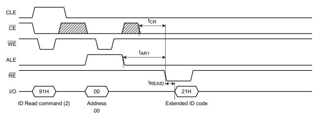
For the specifications of the access times  $t_{\mbox{\scriptsize REAID}},\,t_{\mbox{\scriptsize CR}}$  and  $t_{\mbox{\scriptsize AR1}}$  refer to the AC Characteristics.
