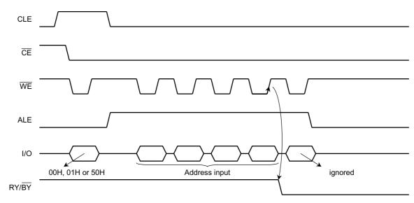
$\overline{\text{WE}}$  Internal read operation starts when  $\overline{\text{WE}}$  goes High in the fourth cycle.
