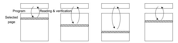
The data is transferred (programmed) from the register to the selected page on the rising edge of -WE following input of the "15H" command. After programming, the programmed data is transferred back to the register to be automatically verified by the device. If the programming does not succeed, the Program/Verify operation is repeated by the device until success is achieved or until the maximum loop number set in the device is reached.
