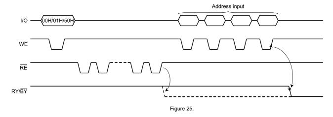
Hence the  $\overline{RE}$  clock input must start after the address input.
