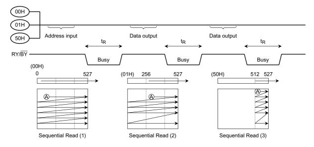
Sequential Read modes (1) and (2) output the contents of addresses 0 to 527 as shown above, while Sequential Read mode (3) outputs the contents of the redundant address locations only.
