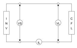
**CFL Testing Circuit**
