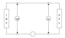
**CFL Testing Circuit**
