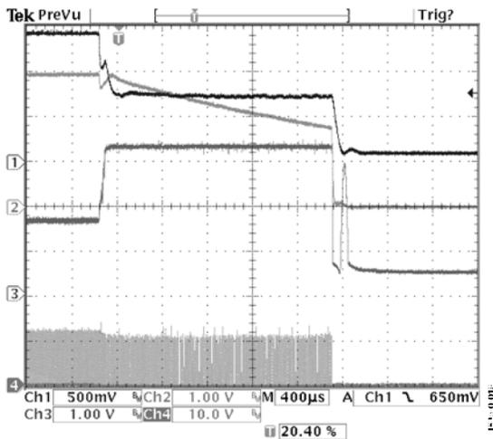
Figure 7. Overcurrent Latch-Off Waveforms
