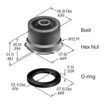
Note: When using boot assembly AT401, also use o-ring AT401P from the standard hardware supplied. Hex face nut AT503 & lockwasher AT508 are not used with boot assembly.
