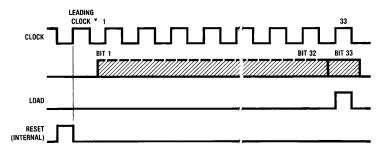
\*This leading clock is necessary only after power ON.
