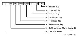
The Periodic Flag Register has the same bit for bit correspondence as Interrupt Control Register 0 except for D6 and D7. For normal operation (i.e., not a single supply application) this register must be written to on initial power up or after an oscillator fail event. D0–D5 are read only bits, D6 and D7 are read/write.
