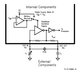
FIGURE 4. Oscillator Circuit Diagram
