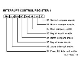
**D0-D5:** Each of these bits are enable bits which will enable a comparison between an individual clock counter and its associated compare RAM. If any bit is a zero then that clock-RAM comparator is set to the "always equal" state and the associated TIME COMPARE RAM byte can be used as general purpose RAM. However, to ensure that an alarm interrupt is not generated at bit D3 of the Main Status Register, all bits must be written to a logic zero.
