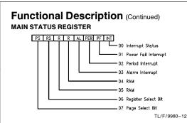
The Main Status Register is always located at address 0 regardless of the register block or the page selected.
