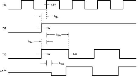
FIGURE 4. Transmit Timing - Start of Transmission
