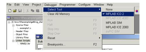
To connect the MPLAB ICD 2, choose <u>Debugger>Connect</u>. See the MPLAB ICD 2 documentation for information on how to configure the MPLAB ICD 2 connection settings.
