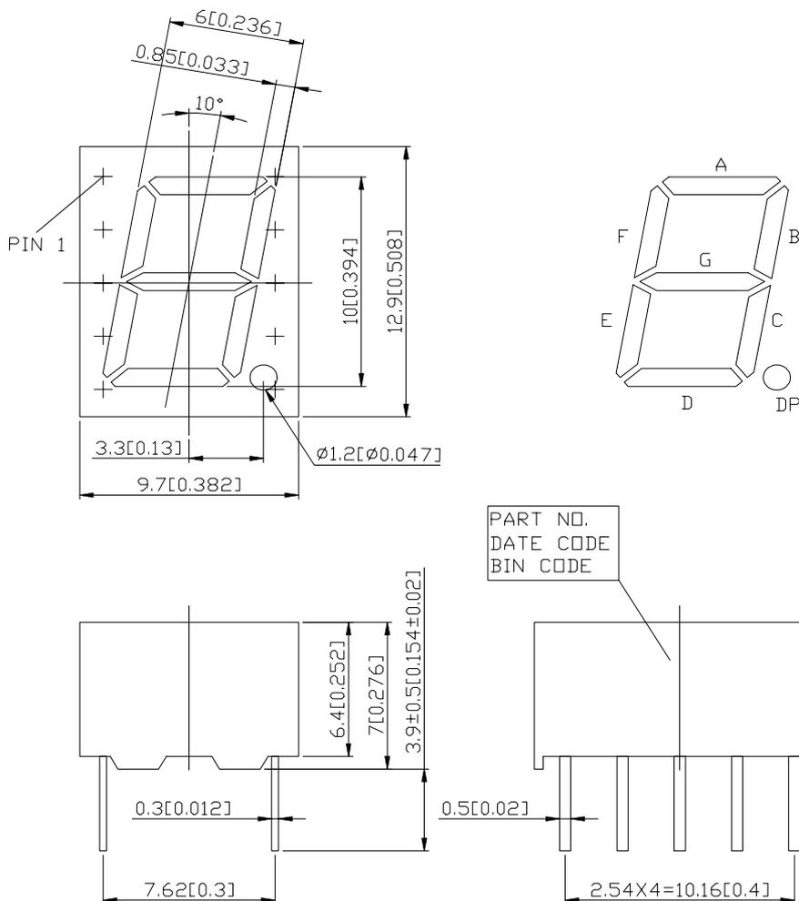
NOTES: All dimensions are in millimeters. Tolerances are ± 0.25 mm (0.01“) unless otherwise noted.
