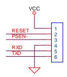
The ISP function uses only six pins: VCC, GND, RXD, TXD, PSEN- and RESET. The simple circuit above is all that must be added to the user's application to use ISP with USB-ICP.
