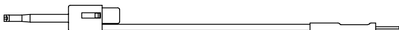
PICO-HOOK, LEAD WIRE DESCRIPTIONS AND COLOR CHOICES: See Basic PICO HOOK. .025" (.635mm) SQUARE PIN PLUG: Gold-Plated Brass Body. Heat Shrink Insulator. Crimp Assembly. See P/N 9265-HS.
