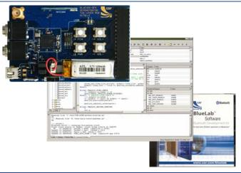
CSR's BlueVOX Flash solution allows you to design high performance, low cost Bluetooth headsets with advanced new software features. Based on the BlueCore4-Audio Flash chip, the new solution combines a high performance, low power Bluetooth radio, 6Mits of on-chip FLASH memory and a comprehensive SDK for complete software flexibility.
