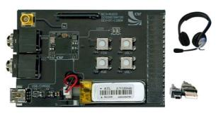
This kit includes all hardware needed to start developing headsets based on the BlueVOX Flash solution, including development PCB, headset and cables and drivers to connect to you PC
