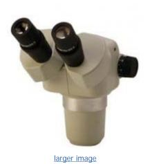
The DSZ-70 Series body can be mounted on a variety of boomstands. You choose the rack & pinion focus mount, illumination, and accessories to meet your specific requirements. Various eyepieces & auxiliary lenses can be used for desired magnification and working distance. Please see our downloadable PDF document below for optical data on the DSZ-Series Microscopes.10x Wide Field eyepieces (field number 20)
