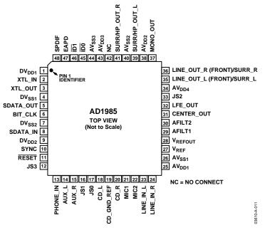
Figure 10. 48-Lead LQFP Pin Configuration
