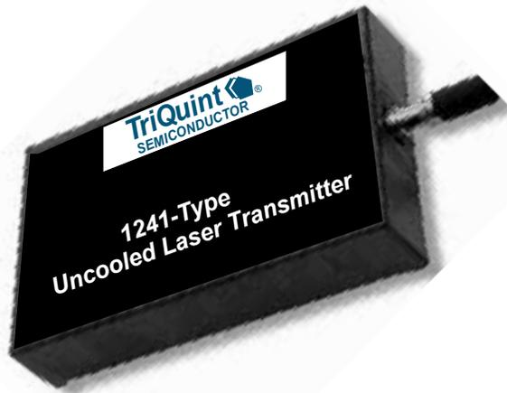
Offering multiple output power options and SONET/SDH compatibility, the 1241/1243-Type Uncooled Laser Transmitter is manufactured in a 20-pin, plastic DIP with a single-mode fiber pigtail.
