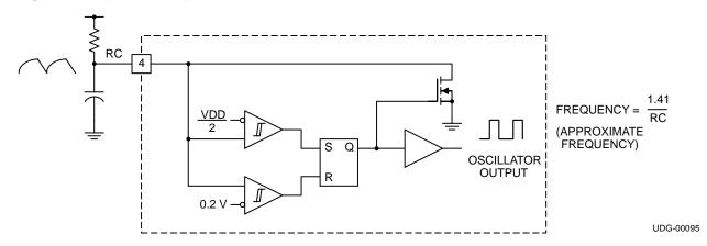
Figure 1. Block Diagram for Oscillator
