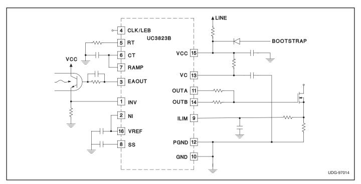
Figure 3. Typical primary side circuit for use with secondary side average current mode controller.
