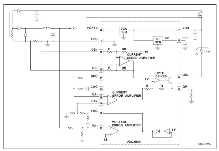
Figure 1. Secondary side average current mode controller.
