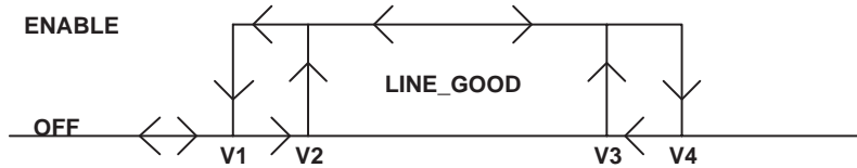
Figure 2. Line UVLO and OVLO Operation
