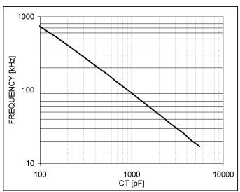
Figure 4. Oscillator frequency vs.  $C_T$  (RT1 = 10k, RT2 = 4.32k)
