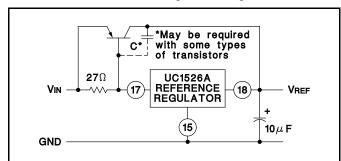
Figure 1. Extending Reference Output Current
