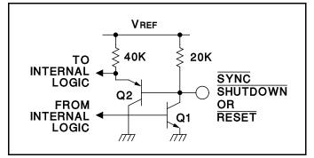
Figure 4. Digital Control Port Schematic
