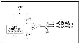
Figure 2. Under-Voltage Lockout Schematic Soft-Start Circuit
