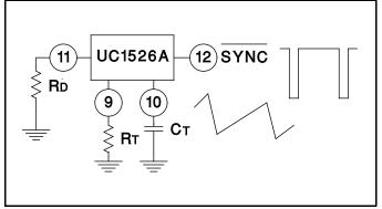
Figure 5. Oscillator Connections and Waveforms
