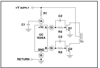
Figure 7. Push-Pull Configuration
