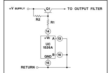
+Vc terminal to ground during switching; however, improved design has limited this cross-conduction period to less than 50ns. Capacitor decoupling at Vc is recommended and careful grounding of Pin 15 is needed to insure that high peak sink currents from a capacitive load do not cause ground transients.
