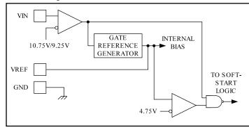
When power is applied to the circuit and VIN is below the upper UVLO threshold,  $I_{IN}$  will be below 600µA, the reference generator will be off, the fault latch is reset, the soft-start pin is discharged, and the outputs are actively held low. When VIN exceeds the upper UVLO threshold, the reference generator turns on. All else remains in the shut-down mode until the output of the reference, VREF, exceeds 4.75V.
