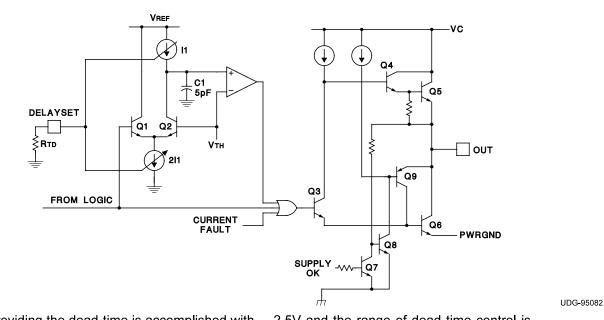
The delay providing the dead-time is accomplished with C1 which must discharge to  $V_{TH}$  before the output can go high. The time is defined by the current sources, I1, which is programmed by an external resistor,  $R_{TD}$ . The voltage on the Delay Set pins is internally regulated to
