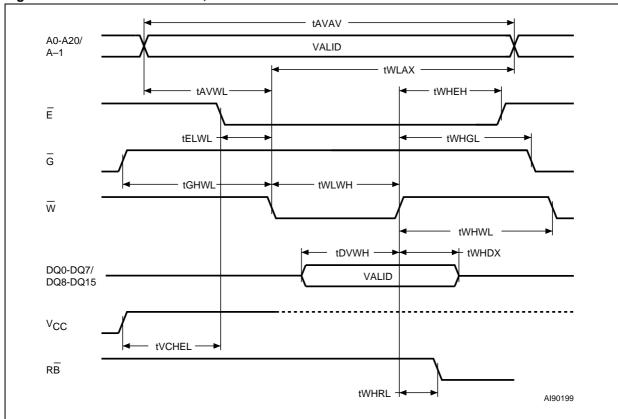
Figure 14. Write AC Waveforms, Write Enable Controlled
