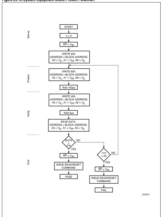
Figure 23. In-System Equipment Block Protect Flowchart
