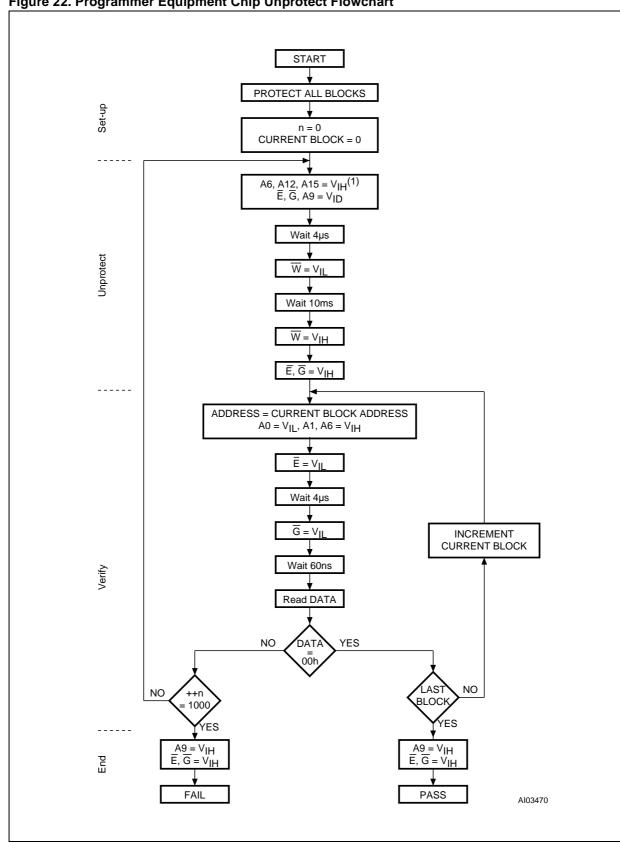
Figure 22. Programmer Equipment Chip Unprotect Flowchart
