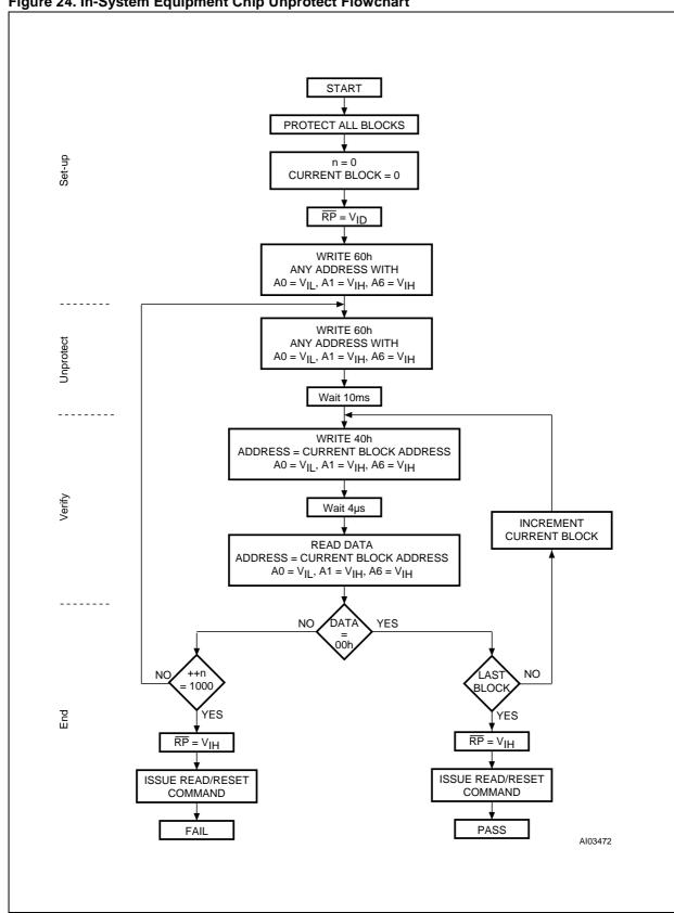
Figure 24. In-System Equipment Chip Unprotect Flowchart
