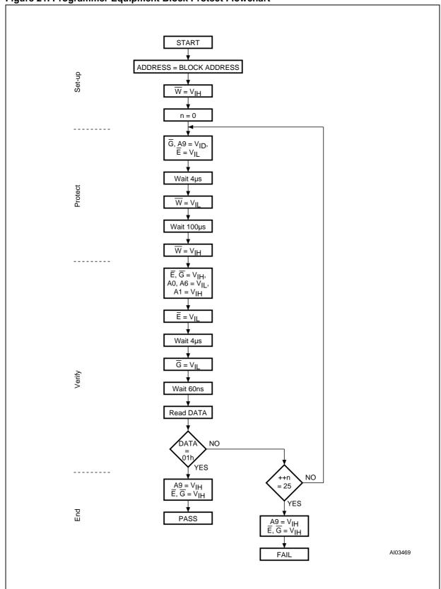
Figure 21. Programmer Equipment Block Protect Flowchart
