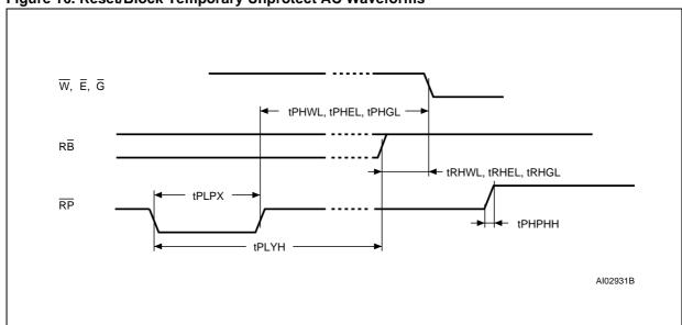
Figure 16. Reset/Block Temporary Unprotect AC Waveforms
