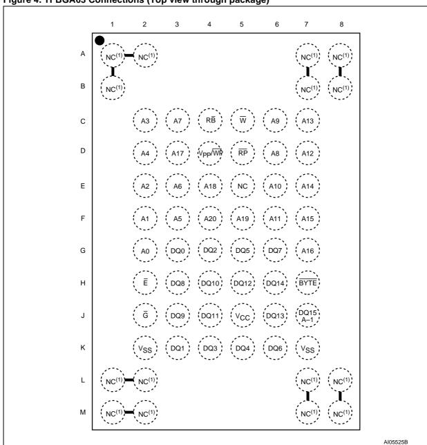
Figure 4. TFBGA63 Connections (Top view through package)
