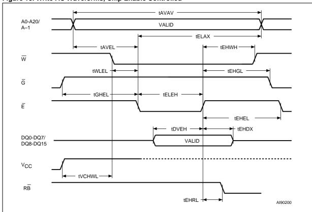
Figure 15. Write AC Waveforms, Chip Enable Controlled
