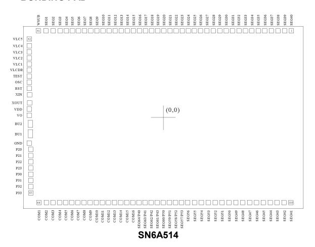
Note: The substrate MUST be connected to Vss in PCB layout.
