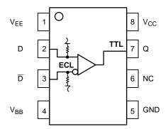
Figure 1. 8-Lead Pinout and Logic Diagram (Top View)
