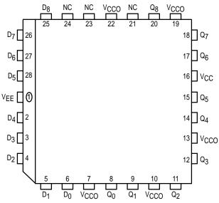
$^{\ast}$  All VCC and VCCO pins are tied together on the die.
