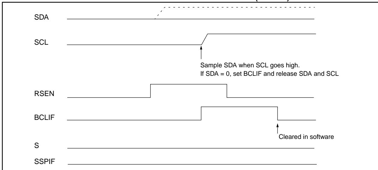
FIGURE 15-42: BUS COLLISION DURING RESTART CONDITION (CASE 2)
