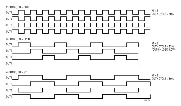
Figure 4. Mulitphase Output Waveforms
