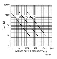
Figure 3.  $R_{SET}$  vs Desired Output Frequency (PH = GND, 2-Phase, M = 1)
