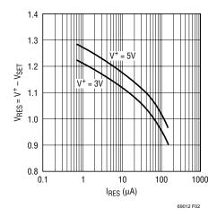
Figure 2. V<sup>+</sup> – V<sub>SET</sub> Variation with I<sub>RES</sub>
