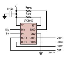
$$f_{OUT} = \frac{10 \text{MHz}}{\text{N} \cdot \text{M}} \cdot \left(\frac{20 \text{k}\Omega}{\text{R}_{SET}}\right); \text{ 5kHz} \leq f_{OUT} \leq 20 \text{MHz}$$
