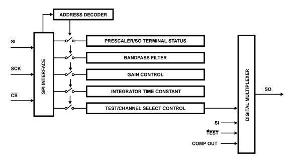
FIGURE 5. PROGRAMMABLE REGISTERS AND STATE MACHINE
