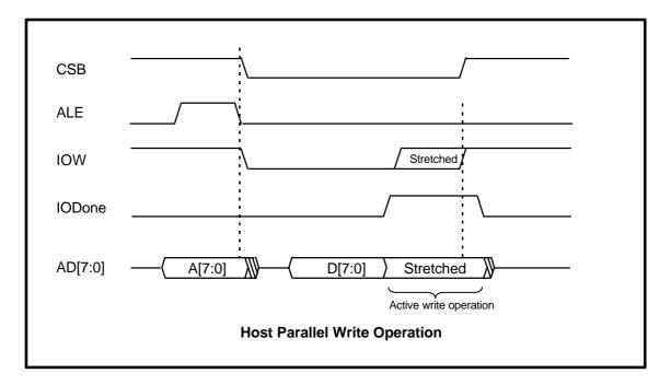
Similar to parallel read operation, parallel write operation needs only 1 operation cycle. The host must watch 'IODone' signal for a proper write operation. IODone signal indicates the completion of read/write operation. So the host must hold the IOW, CSB, Write Data[7:0] signals until IODone signal become active. When IODone signal become active, ISP accept the write data internally. At the final stage, the host ends the bus cycle(CSB, IOW, Write Data[7:0]) and IODone signal become inactive.
