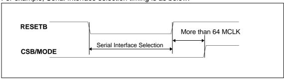
For example, Serial Interface selection timing is as below.
