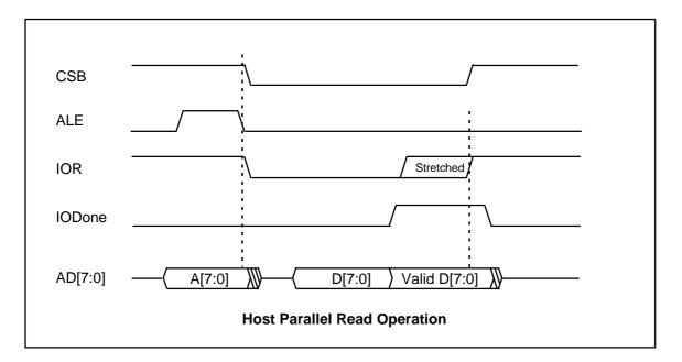
A Parallel read operation always needs only 1 read cycle different from the serial read operation. But the host must watch 'IODone' signal for a proper read operation. IODone signal indicates the completion of read/write operation. So the host must hold the IOR, CSB signals until IODone signal is active, to read the valid data on AD[7:0] lines. At the final stage, the host ends the bus cycle(CSB, IOR) then IODone signal become inactive.
