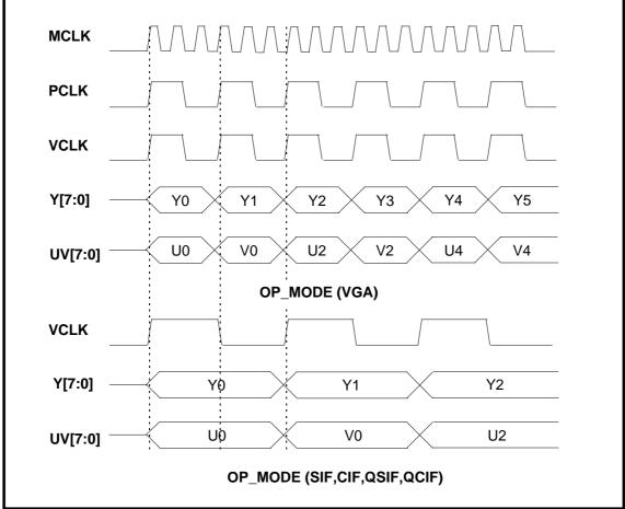
\* Note : HV7131B(VGA) CMOS Sensor is used for this timing diagram.
