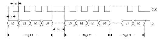
• Data latch timing for 5-bit pattern (MODE=1)
