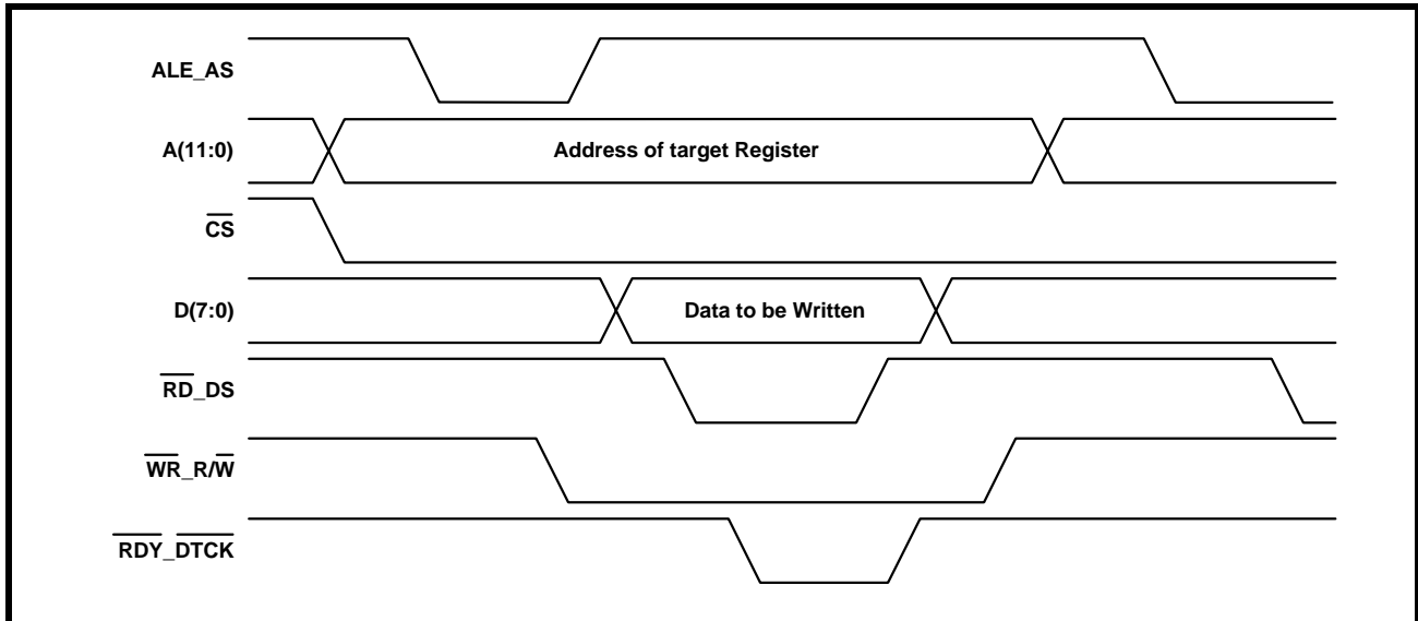
FIGURE 28. ILLUSTRATION OF THE BEHAVIOR OF THE MICROPROCESSOR INTERFACE SIGNAL, DURING A MOTOROLA-TYPE PROGRAMMED I/O WRITE OPERATION
