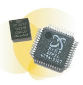
The chipset consists of the GSP2t, highly integrated digital chip, GRF2i/LP integrated RF receiver and the SiRFNav software. The GSP2t is packaged as 7mm 48 pin LQFP packages and the GRF2i/LP is in a 5mm 32 pin QFN package. External components are minimized thanks to their high level of integration. SiRFNav software is designed for easy porting to most common host systems.
