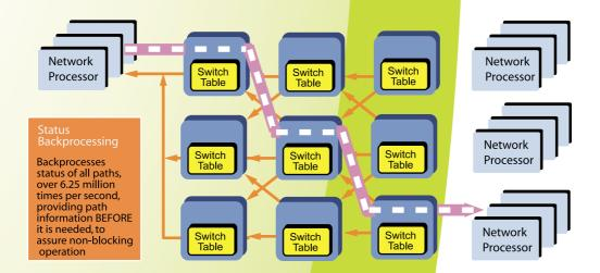
Tremendous Scalability and Power - The GES0016 switch fabric ICs can be clustered to give non-blocking switch fabric performance for the GEP2C02 Network Processors providing wire speed Layer 2-7 switching in configurations ranging from 32 Fast Ethernet Lines to 128 Gigabit Ethernet Lines.
