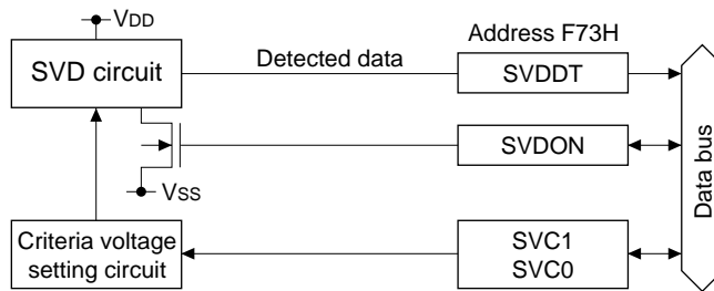
Fig. 3.2.1.1 Configuration of SVD circuit
