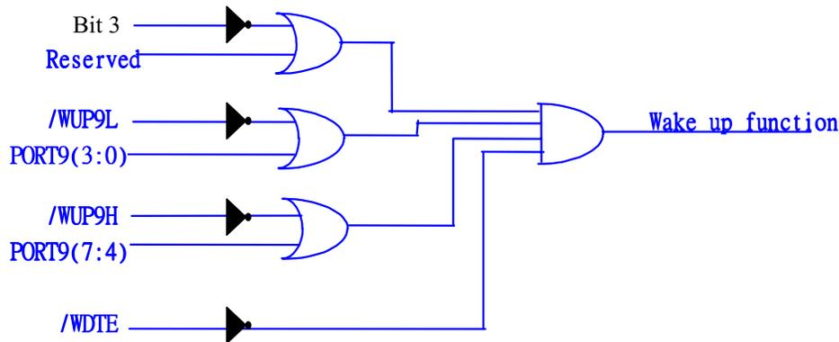
fig.9 Wake up function and control signal
