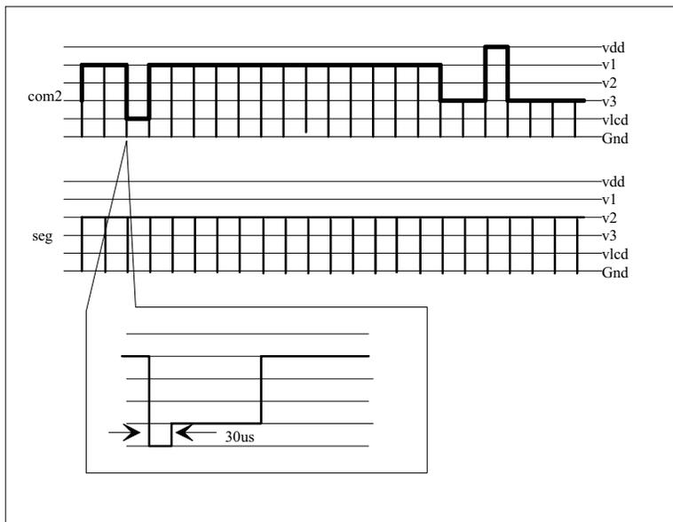
Fig.11.key scan signal
