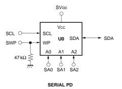
Remarks 1. Rambus Channel signals form a loop through the RIMM module, with the exception of the SIO chain.2. See Serial Presence Detection Specification for information on the SPD device and its contents.
