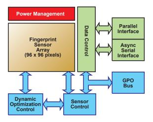
The FingerLoc AFS8500 sensor incorporates flexible SelectaBus architecture, allowing the developer to deploy designs that use either the familiar asynchronous serial interface or an 8-bit parallel interface implementation.
