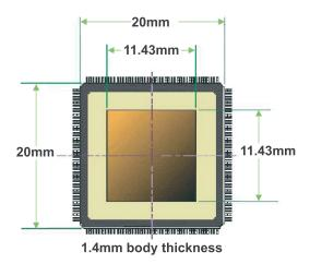
The form factor of the FingerLoc AFS8500 is 144-pin JEDEC-standard Low-profile Quad Flat Package (LQFP)
