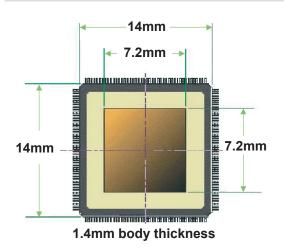
The form factor of the EntréPad AES3500 is 100-pin JEDEC-standard Low-profile Quad Flat Package (LQFP)
