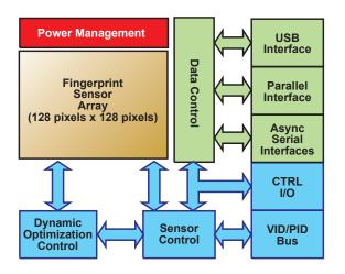
The EntréPad AES3500 sensor incorporates flexible SelectaBus architecture. This feature allows the developer to deploy designs that use not only the popular Universal Serial Bus, but also asynchronous serial interfaces and an 8-bit parallel interface implementation.
