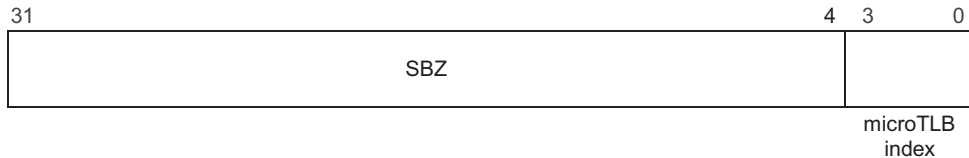
Figure 3-18 MicroTLB index format
