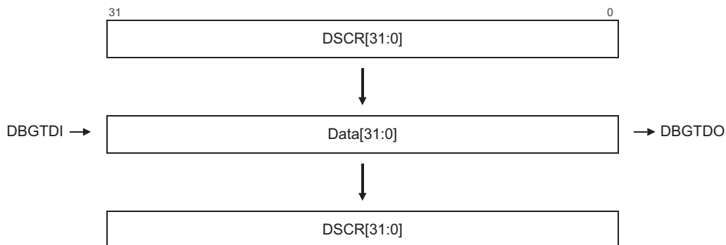
Figure 14-8 Scan chain 1 bit order
