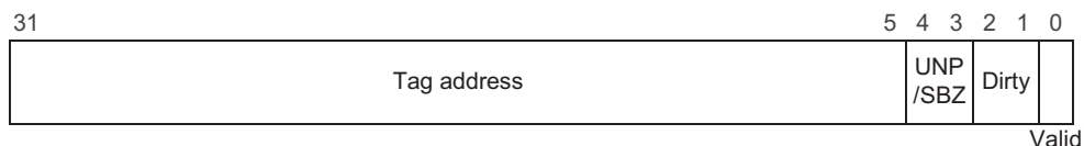
Figure 3-16 Instruction and Data Debug Cache Register format
