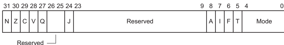
Figure 3-1 Program Status Registers
