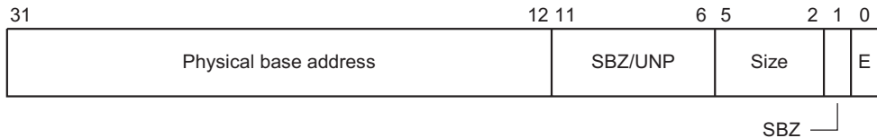
Figure 3-21 DTCM and ITCM Region Registers
