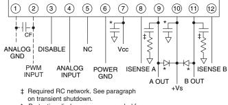
Protection diodes are recommended for applications where +Vs exceeds 50V.
