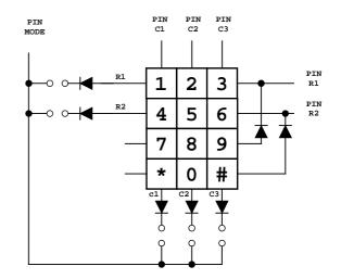
Double contacts under keys 0-9\*#: One contact is connected to AS2504, the other one to CPU.
