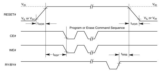
Figure 23. Temporary Sector Unprotect Timing Diagram
