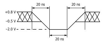
Figure I. Maximum Negative Overshoot Waveform
