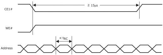
**Note:** The S71JL064HA0 Model 61 has a timing that is not supported at read operation. Data will be lost if your system has multiple invalid address signal shorter than  $t_{RC}$  during over 15 $\mu$ s at the read operation shown above.
