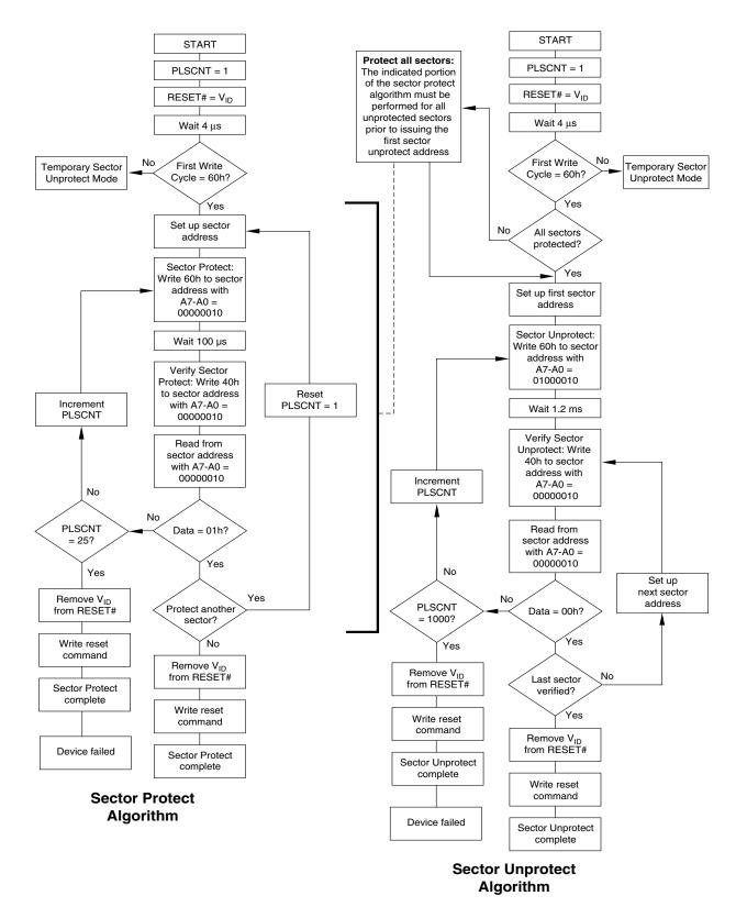
Figure 3. In-System Sector Protection/Sector Unprotection Algorithms
