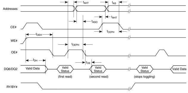
Figure 20. Data# Polling Timings (During Embedded Algorithms)
