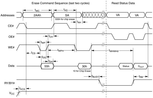
1. SA = sector address (for Sector Erase), VA = Valid Address for reading status data (see "Write Operation Status"
