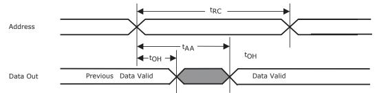
**Note:**  $CE1\# = OE\# = V_{IL}$ ,  $CE2 = WE\# = V_{IH}$ , UB# and  $OF LB\# = V_{IL}$
