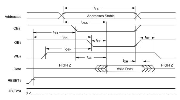
Figure I3. Read Operation Timings
