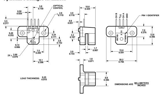
$Mounting\ Option\ \#51-Screwmount\ (Baseplane\ Mounting)$
