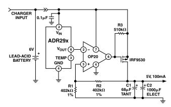
Figure 8. Voltage Regulator for Portable Equipment
