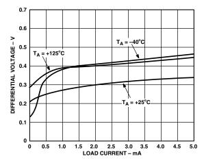
TPC 10. ADR290 Minimum Input-Output Voltage Differential vs. Load Current
