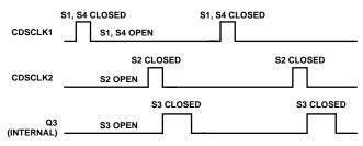
Figure 9. CDS-Mode Internal Switch Timing
