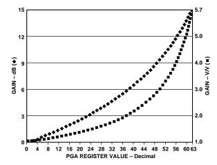
Figure 13. PGA Gain Transfer Function
