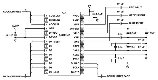
Figure 14. Recommended Circuit Configuration, 3-Channel CDS Mode
