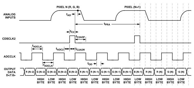
Figure 3. 3-Channel SHA Mode Timing
