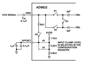
Figure 8. CDS-Mode Input Configuration (All Three Channels Are Identical)
