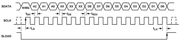
Figure 7. Serial Read Operation Timing
