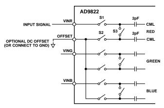
Figure 10. SHA-Mode Input Configuration (All Three Channels Are Identical)
