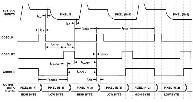
Figure 2. 1-Channel CDS Mode Timing
