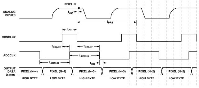
Figure 4. 1-Channel SHA Mode Timing
