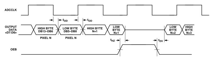
Figure 5. Digital Output Data Timing
