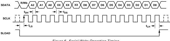
Figure 6. Serial Write Operation Timing
